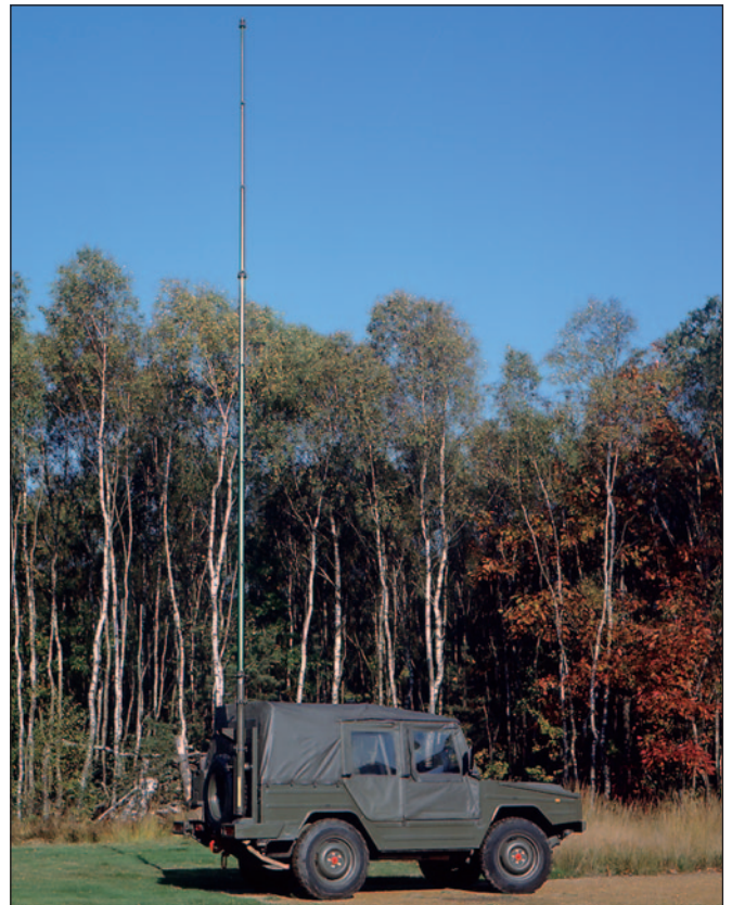
Photo: PU Mast vehicle mounted, unguyed.
