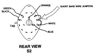
Use a cutoff lead from a resistor or cap for these jumpers. Solder the jumpers at lugs 4, and 5, but do NOT solder lug 7 yet..
